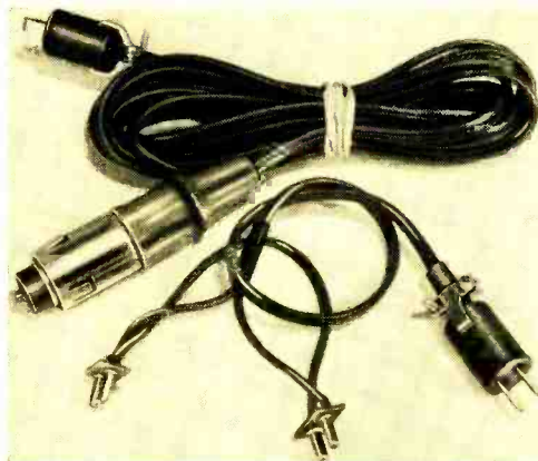
Fig. 7. Alternate cables permit powering amplifier from batteries or car cigarette-lighter receptacle.
