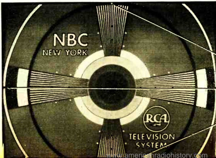
Fig. 1. Typical test pattern transmitted by television stations. Note parallel edges, square corners.
