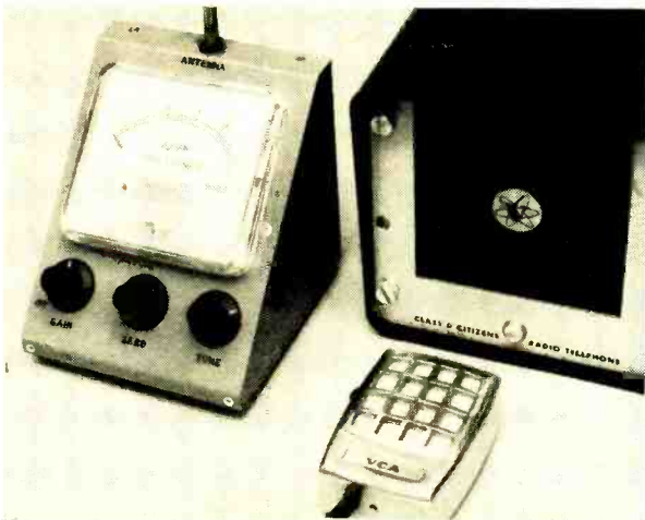
Lafayette field strength meter has built-in single-transistor amplifier. Right-hand control broadly tunes the input circuit.
