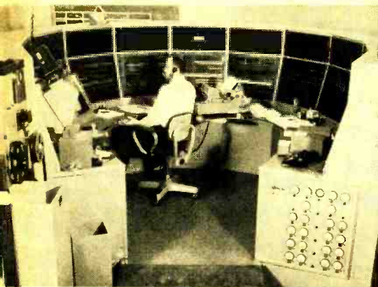
This computer at Lincoln Laboratory analyzed 10,000,000 computations to confirm existence of weak radar echoes from Venus.
