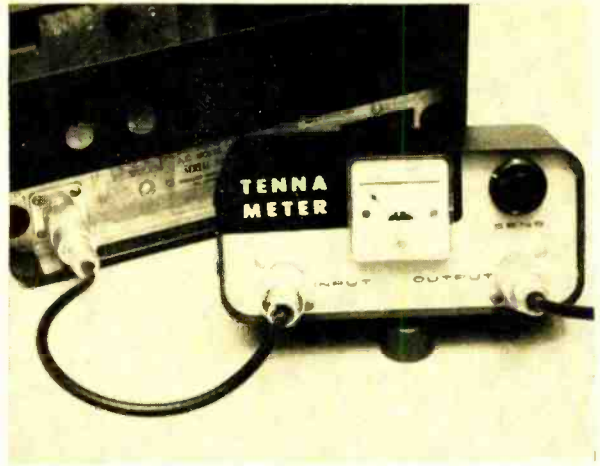
Globe output meter serves as monitor and modulation check. It is left in transmission line at all times.
