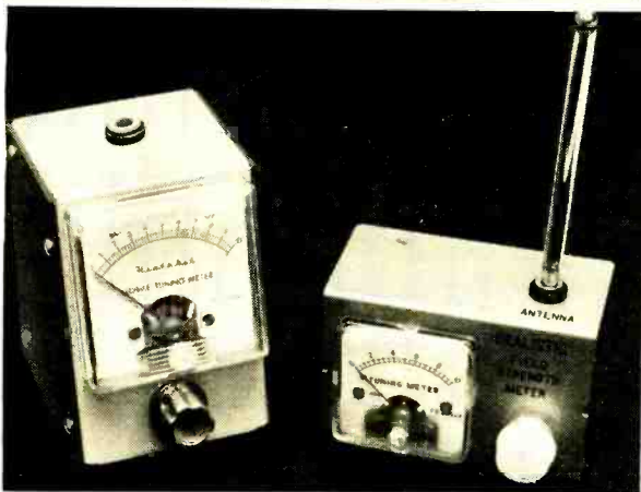
Heathkit and Radio Shack field strength meters have magnets in underside of case to hold meter to automobile steel dashboards.
