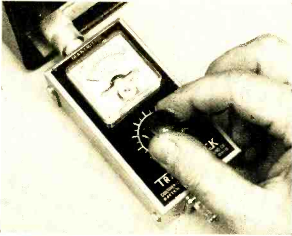
CESCO Transicheck measures output power in watts, and may be used to check on feed line efficiency.
