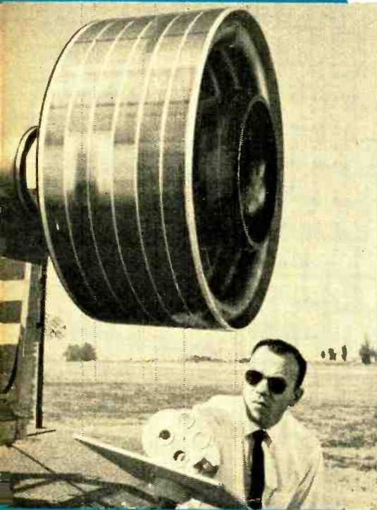
Spinning satellite, built by Hughes Aircraft, is an "active" repeater. It weighs 32 pounds and is powered by silicon cells.
