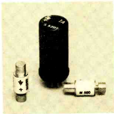
Packaging of diodes in tube shells permits replacement of 5U4, 5W4, 5Y3, 6X4 and other rectifiers. Cartridge-cased diodes are used in the newer TV sets.
