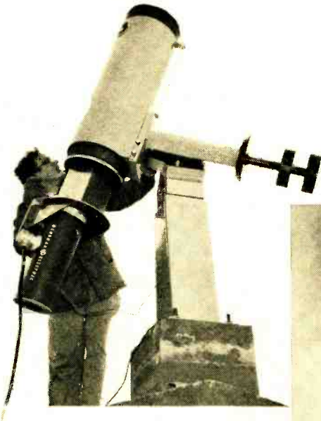
Two methods of satellite tracking. At right is the new 33-element helical beam antenna at Wallops Space Flight Station. Above is General Electric's optical tracker using a high-power telescope and special TV image pickup tube.
