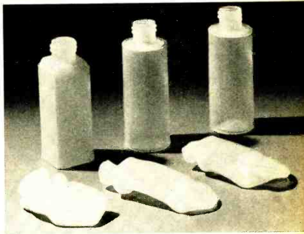
Irradiated polyethylene bottles (top), comprised of "cross-linked" molecules, can withstand prolonged exposure to temperatures as high as 250° F. Non-irradiated bottles (bottom) wilt to shapeless blobs.
