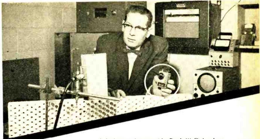
A dosimeter developed by Dr. A. W. Richardson of Saint Louis University is used to measure r.f. radiation. Worn by a maintenance technician, it sounds an audible tone when r.f. intensity becomes dangerous.
