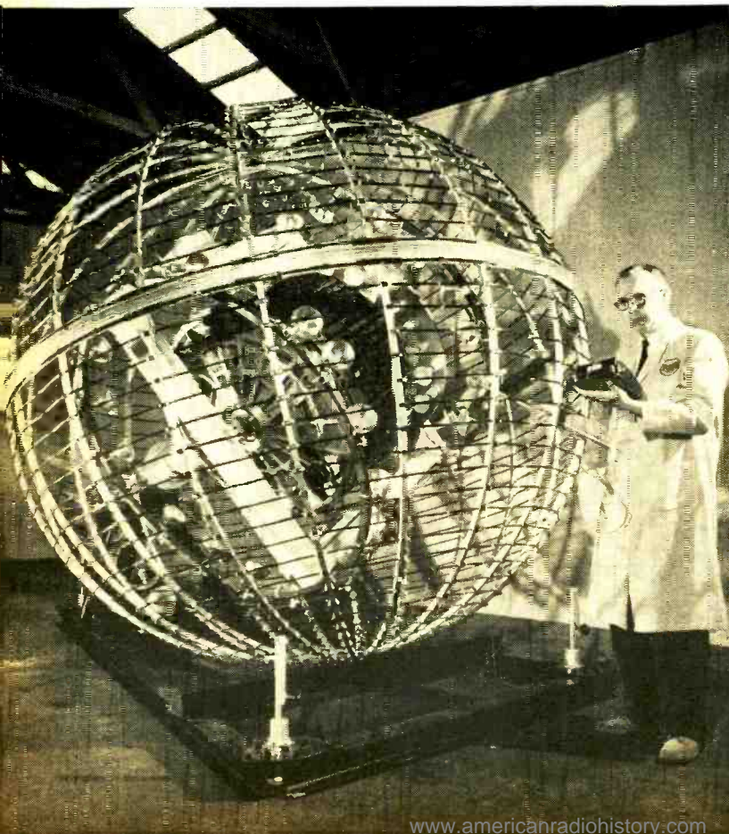
Spherical "cage" designed to produce magnetic fields resembling those of the earth was used in pre-launching tests of Tiros II. Here, Warren P. Manger, of the RCA Astro-Electronics Division, takes reading of magnetic effect within the wired "cage," preparatory to rotating the satellite on its mount for study of the orientation system.
