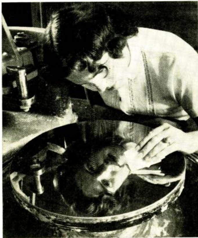
Infrared “picture window” produced by scientists at Hughes Aircraft is solid germanium casting 15” in diameter and 1/2” thick. Optically ground and polished, it is opaque to ordinary light but refracts infrared rays much as a glass lens collects and focuses rays from visible part of spectrum. Used in missile detection systems, the casting is made from 9½ pounds of germanium, and is valued at approximately six thousand dollars.
