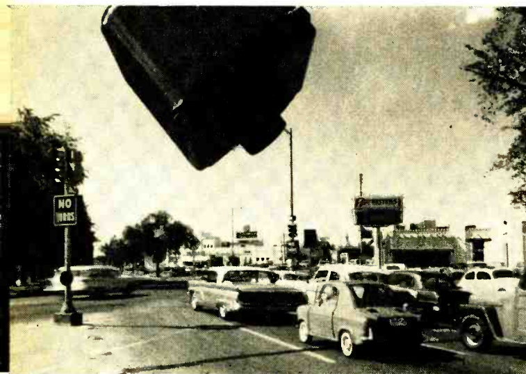
Traffic detector —the "Traffitrol"—uses infrared beam to detect and count vehicles traveling at speeds up to 80 miles per hour. Highly accurate and virtually foolproof, the device is among the first to apply infrared principles to traffic problems. The "Traffitrol" is manufactured by the Heiland Division of Minneapolis-Honeywell.
