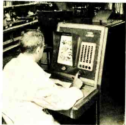
"Autotutor," made by U. S. Industries, includes unit (on top) which records the length of time a student takes to answer a question as well as the answer he chooses.
