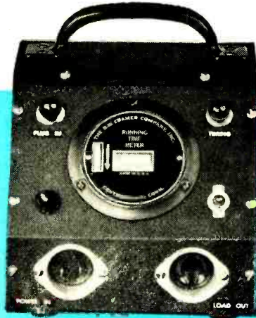
Job timer is mounted in sloping front cabinet; power plugs mount on front apron.
