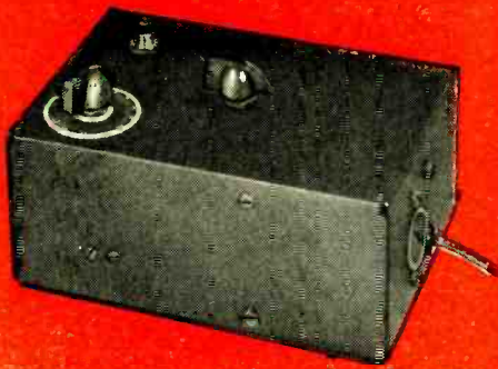
Photo timer controls mount on top of cabinet; R3 has timing scale (white circle).
