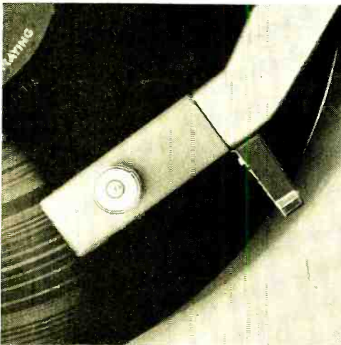
Adjusting cartridge shell to make it parallel with record surface is easy with a circular level. Some pickups can also be adjusted from side to side.
