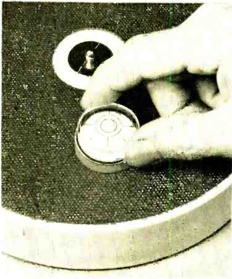
Circular bubble level costs about 90 cents, can be placed anywhere on turntable, and will reveal even small amounts of slope without repositioning.
