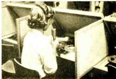
Student's booth contains a tape recorder, a microphone, and a set of headphones. The student listens to a prerecorded lesson and repeats it phrase by phrase into his tape recorder. In playback, he hears the two tracks one after the other and is able to compare his pronunciation with that of the instructor.
