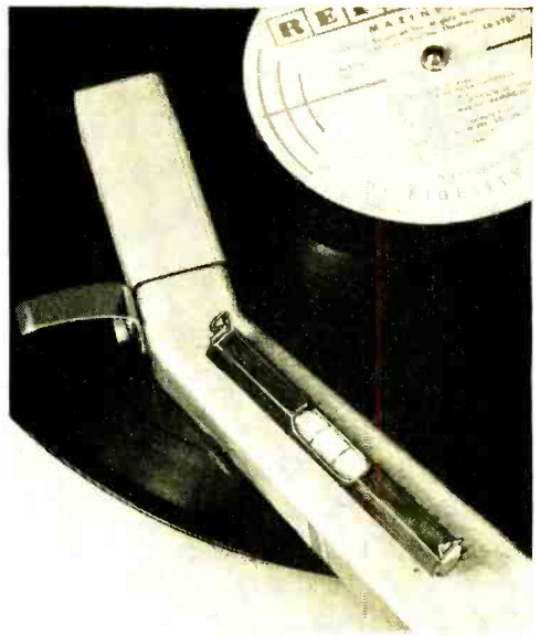
Top surface of most professional tone arms should be parallel to the record surface. Check this with a level and adjust height of the arm accordingly.
