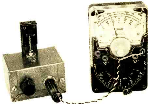
Tunnel-diode transmitter is adjusted with external multimeter to determine the diode's negative-resistance region.
