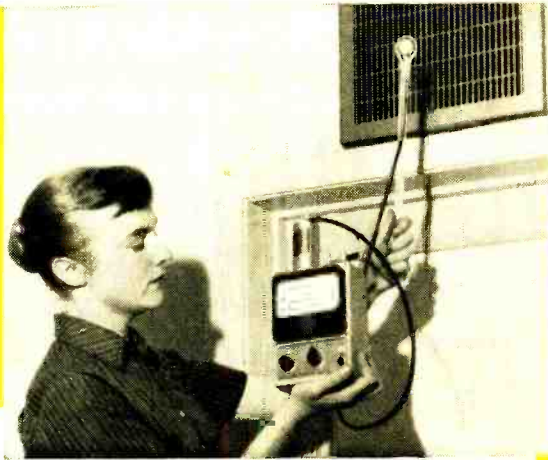
Using a Keithley electrometer and Beckett probe to detect presence of ionized air. Here, this device will determine if the air conditioner is sending ionized air into the room.
