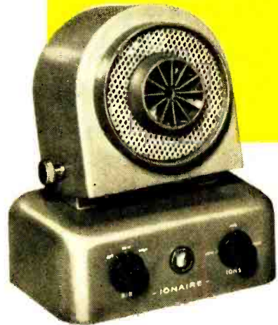
A simple device for producing and controlling negative ions in a closed room, the Wesix Ionaire consists of a rectifier and a piece of radioactive tritium foil mounted within a conducting tube.
