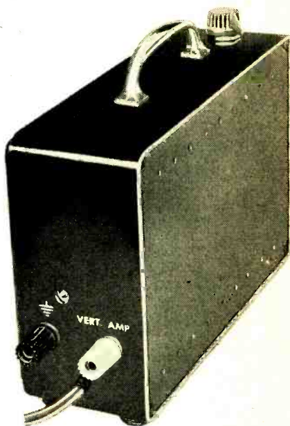
Completed scope is compact and fully portable. Rubber feet on bottom protect case; holes on side were added for ventilation.
