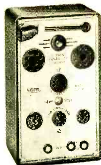
Fig. 1. A continuity checker, such as the EICO Model 612, is among the simplest types of tube testers. Helpful in tracking down tube troubles, it has a pilot lamp which will light if tube filaments or heaters are okay.
