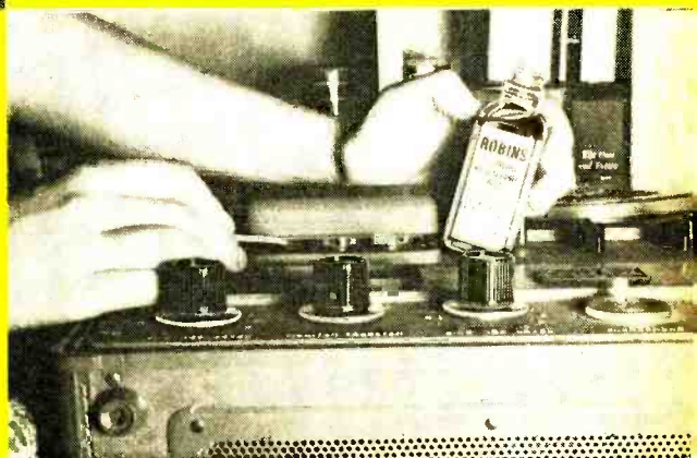
Speedwinders cut rewinding time. This one, the Heath SW-1, handles 10½" reels and rewinds 1200' of tape in 40 seconds.
