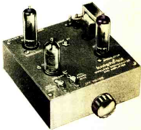
Versatile Knight-Kit wireless broadcaster/amplifier can be used with almost any phono pickup or microphone. Signals can be broadcast or fed directly to a speaker.
