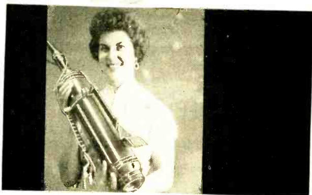
This is the custom-built TV camera that sends back pictures from the bottoms of deep wells.
