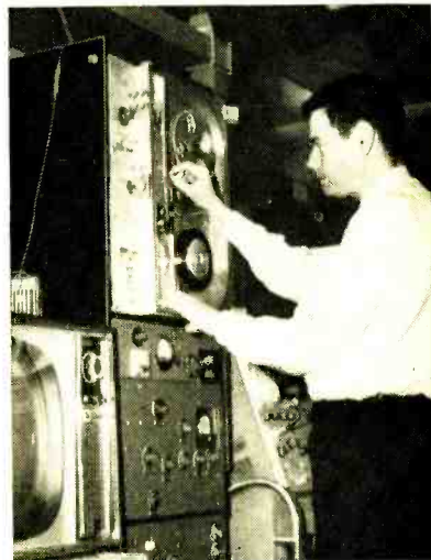
Dr. Glenn tests his prototype thermoplastic recorder. He estimates that he could halve its size by rebuilding it. Diagram of the TPR recorder is at left.
