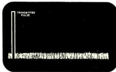
Fig. 4. On conventional radar, thermal noise completely swamps out echoes of low amplitudes.
