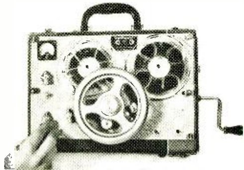
Spring-wound motor is employed by Amplifier Corp. of America's Model 612-TD. This precision-made recorder is intended for use in remote areas where extra batteries are not available.
