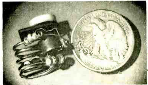
Fig. 3. Simple FM transmitter circuit featuring the new "tunnel" diode.
