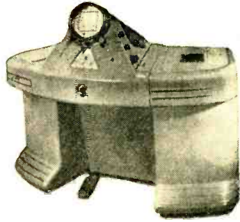
Two of the most widely used electron microscopes are shown here. At left is the RCA EMU-3, capable of 200,000X magnification. Above is the Norelco EM100B, which magnifies to 90,000 times.
