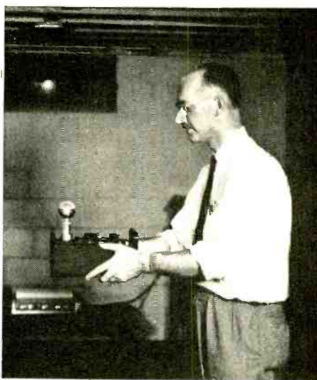
Professional sound-measuring instruments were necessary to obtain data on the results of installing various amounts of acoustical tile.
