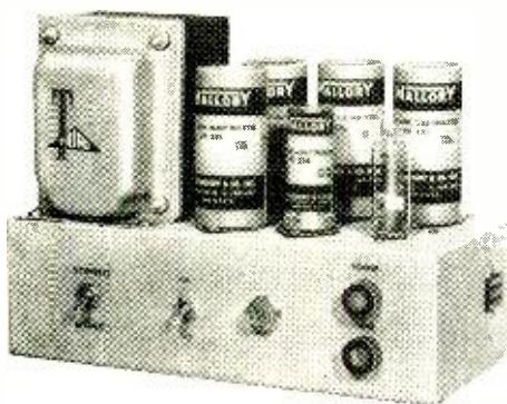
Power transformer T1 shown in schematic diagram of power supply is RCA type with dual filament windings. Triad model has single winding.
