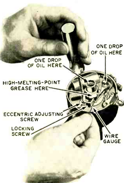
Fig. 8. Points are adjusted for proper gap width with a screwdriver and a wire gauge. See text for details.
