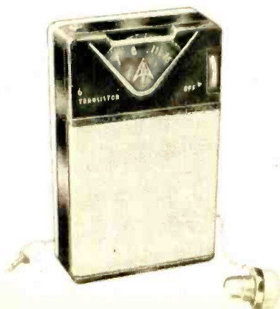
Personal-sized six-transistor receiver now available from Argonne features push-pull output to its built-in PM loudspeaker.
