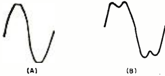
Fig. 12. Slight (A) and extreme (B) clipping which occurs when output stage of amplifier is overdriven.
