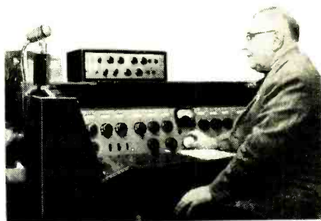
Audio console is "brain" of the TV audio operation. As well as mixing and controlling the many mikes, it can also be used to add reverberation and other special effects to audio portion of show.
