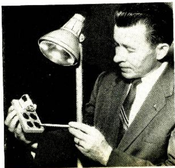
Solar energy demonstration kit developed by Hoffman Electronics Corp. can be used with standard lamp bulb.
