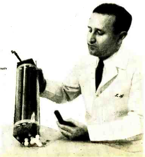
Fig. 1. Operation of the fuel cell. Electron flow from hydrogen electrode to oxygen electrode provides electric current.
