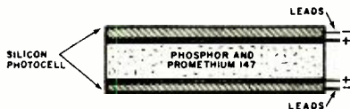
Fig. 5. Promethium cell composed of center layer of promethium and phosphor with outer layers made up of photocells.
