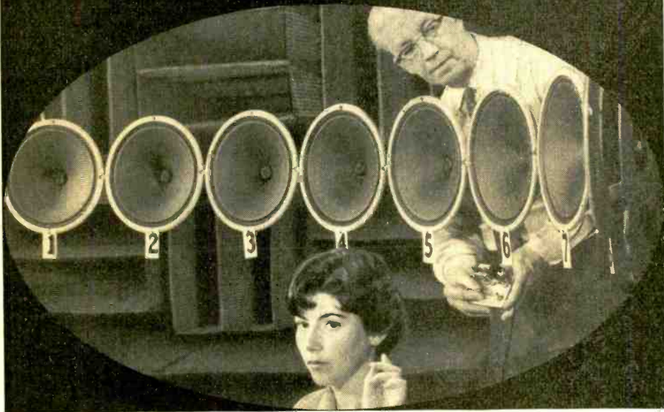
Which speaker is making the sound? In echoless chamber at Bell Labs, Robert Hanson measures test subject's ability to localize sounds — observes how two ears operate in partnership. This and other tests may point the way to better telephone instruments.
