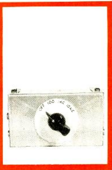
TRANSISTOR SQUARE WAVE GENERATOR —This is an easily constructed piece of test gear that has many applications to the audio field. You'll find it's an efficient, cheap way to test circuits and amplifiers.
