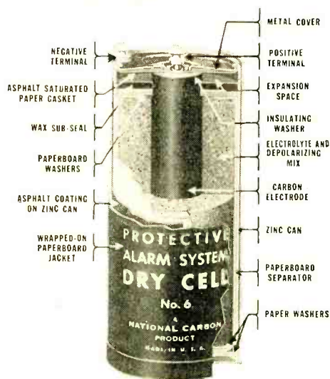
Fig. 1. Cross-section view of a typical dry cell.
