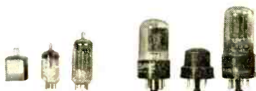
The "active" elements in the VTVM. Standard models usually have a lineup comprising (from left to right) a 50-ma. power supply selenium rectifier, a 6AL5 a.c. rectifier and a 12AU7 bridge tube. An alternate arrangement consists of a 6X5 power rectifier, a 6H6 a.c. rectifier and a 6SN7 bridge tube.
