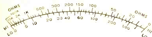
Fig. 7. Comparison of series- and shunt-type ohmmeter scales. LO is the shunt scale, HI the series scale.
