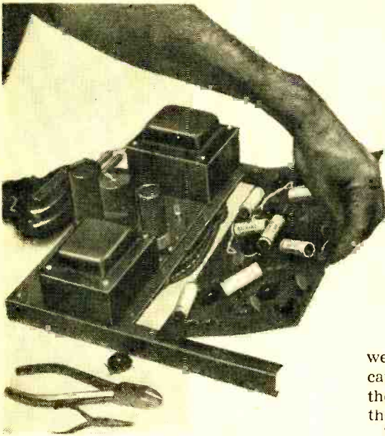
Printed-circuit board is wired as a unit and is installed on chassis when power supply has been completed.
