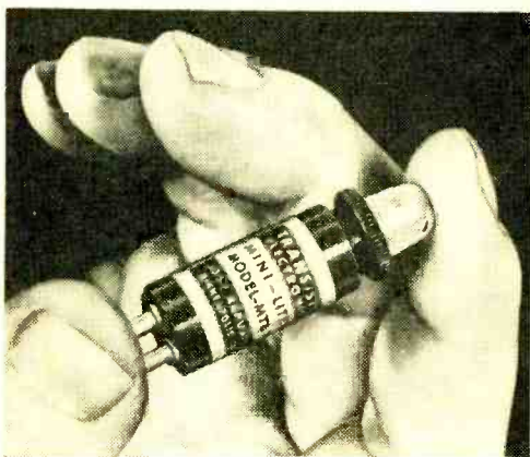
Tiny transistorized panel display light, the "Mini-Lite," made by Transistor Electronics Corporation.
