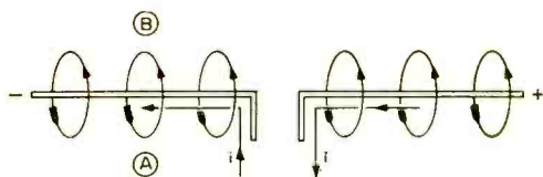
Fig. 3. Magnetic field surrounding the half-wave dipole takes the form of concentric circles lying in planes perpendicular to the conductor.
