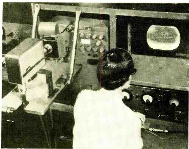
Fig. 2. Special setup used by Philco's Lansdale Tube Company Division to test ultra-high-speed switching transistors with very short rise time. The TW oscilloscope, made by Edgerton, Germeshausen & Grier, Inc., has an inherent rise time of only 0.1 millimicroseconds. Transistor waveforms are checked on television screen as shown in photo.
