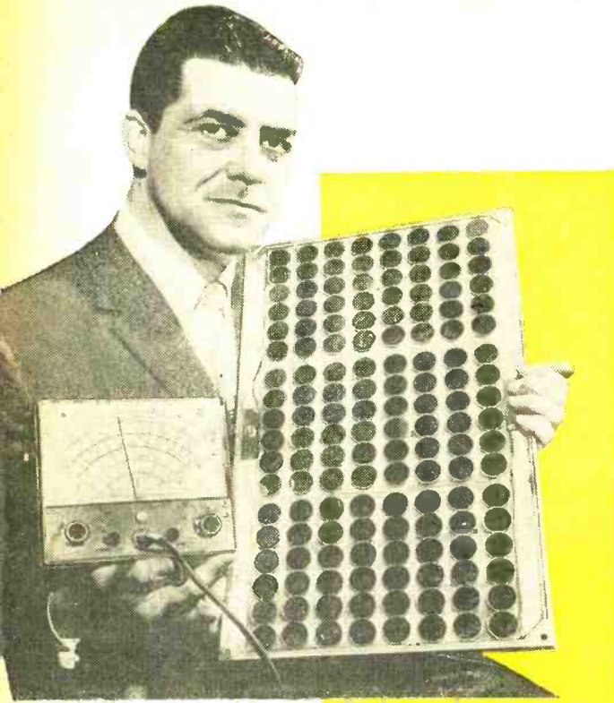
A series-parallel combination of 144 Hoffman silicon solar cells will supply five watts of power to a 6-volt battery system in bright sunlight.
