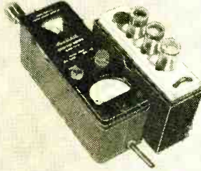
GRID DIP METER
