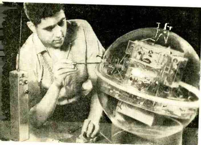
The designer of the satellite is shown at left making an adjustment in an equatorial thermistor sensor which registers skin temperature. Above is a view of the “works” in Argus I. Note that almost all components are cased in plastic to allow full visibility—the metal box at bottom houses the “Brain”. Diagram below shows frequencies used by satellite.
