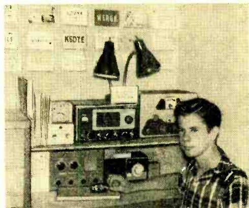
Mike, KN6KZD, runs 75 watts to his new Heathkit DX-40 on 80, 40 and 15 meters. His receiver is a Hallicrafters S-53A. Mike QSL's 100%.
