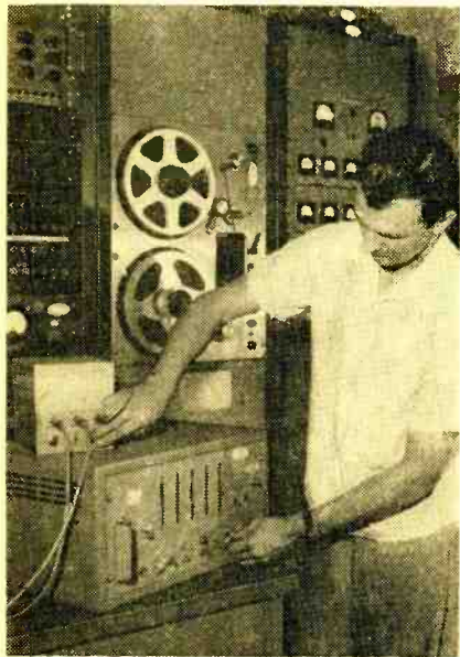
Tape speed indicator at RCA center is adjusted by technician before missile launching.
