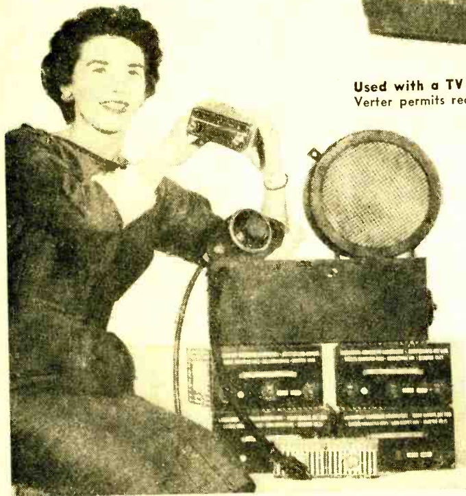
The young lady above is holding a new all-transistor auto-portable receiver which may be used either in or out of an automobile. Compare this in size with the 1929 Cadillac auto radio shown with its B batteries.
