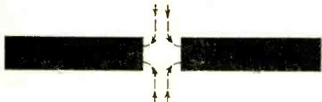
Fig. 7. The same effect is shown here as in Fig. 6 except that both sets of lines have been reversed in direction by turning them end over end.
