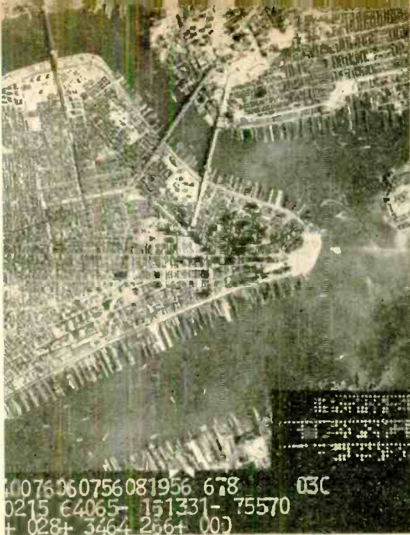
A camera writes its own captions! The illustration above shows how position, altitude and other pertinent data necessary to Air Force reconnaissance can be recorded automatically on photos. Developed by Federal Telecommunication Labs, the Digital Data Recording Device records all data in coded dot form (lower right on photo). During development, a ground-based reader decodes and prints data under picture.
