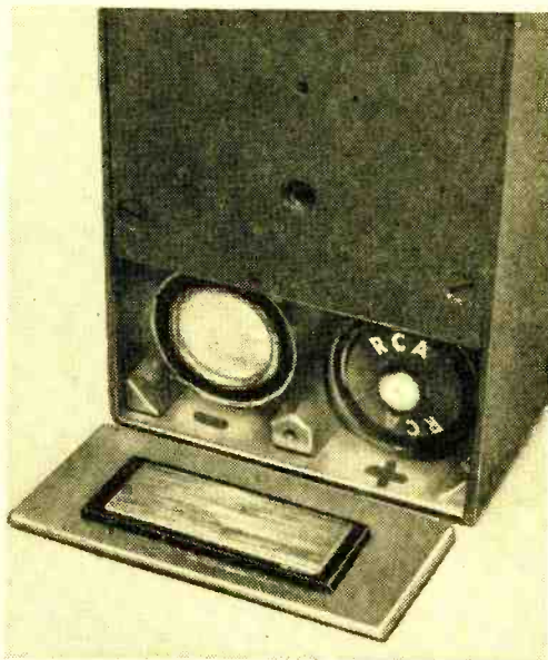
Battery installation; note the polarity markings and insulated contact plate.
