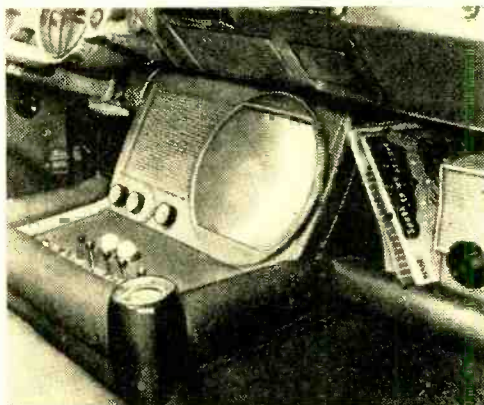
Control panel of car uses TV channel selector.
