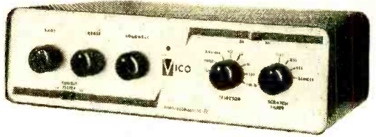
▲ A real innovation is this first all-transistor amplifier by Vico. The use of transistors virtually eliminates hum. Output is 20 watts.
