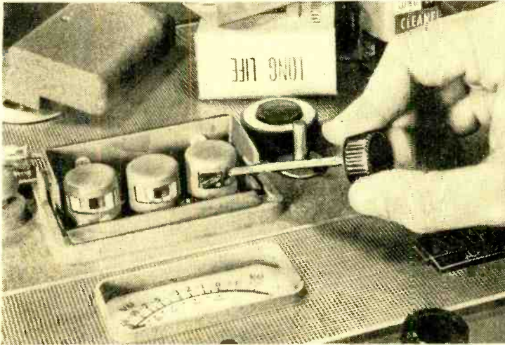
Recording heads may be cleaned with a special cleaning fluid which dissolves binder and oxide deposits that build up near the magnet gap. Despite its solvent quality, the fluid doesn't attack metal or plastic parts of the recording head.
