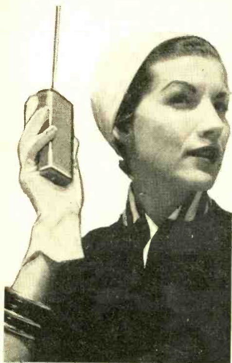
The little lady above is shown demonstrating one-way radio paging. Subscriber presses button and hears the taped message.
