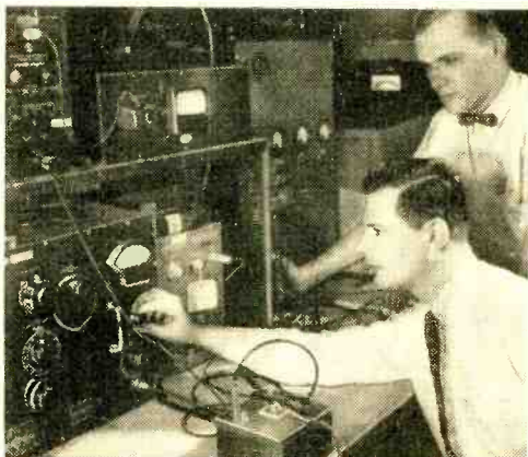
Experimental power transistors at Bell Telephone Laboratories, such as the silicon unit being checked here, can provide a 5-watt output at 10 mc.
