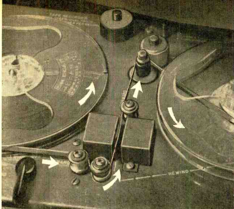
Arrows show path of tape from feed to take-up reels during recording. Note that on this particular machine an alternate path is required for rewind of tape. Each roller and its pad, around which tape passes, must be in good working condition for best results.
