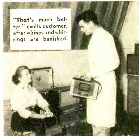
"Your trouble is flutter" says the audio expert, checking phonograph with "Wow and Flutter Meter."
