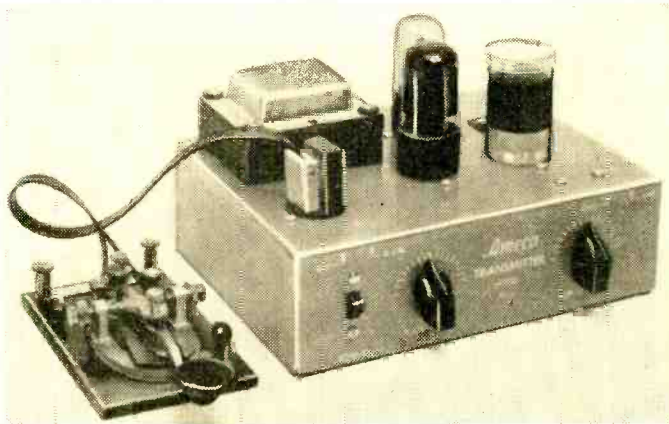
Kit transmitter (AMECO AC-1) assembled by author (key not supplied).
