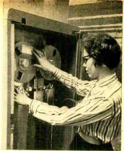
Loading reels or running the tape “reader” (above) merges clerical and technical job categories even at ground-floor level. At the N. Y. Life Insurance Co., electronic data storage saved space equivalent to four basketball courts.
