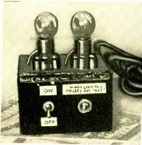
"Worm-Turner" No. 1 , complete with a.c. power cord. Incandescent bulbs limit current flow through earth probes. Neon lamp, to right of switch, indicates when probes are "hot" and ready for use.
