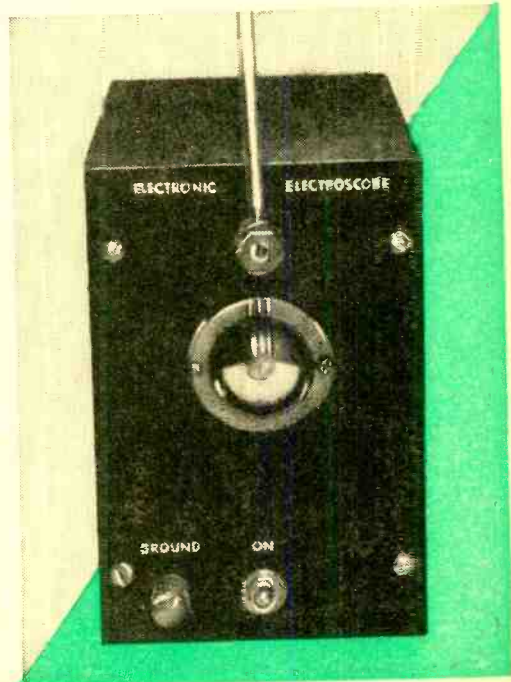
Rubbing an insulator with soft cloth and bringing it near the feeler antenna of the electroscop will close its "eye." This unit can take a 100,000-volt discharge safely. The chassis is welded to front panel of case, shown below.
