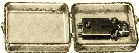
Vibration pickup or "transducer" assembly; crystal phono cartridge is mounted in small plastic case.
