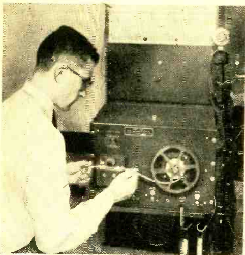
At WIAW, the operator adjusts the tape transport mechanism for the daily code lessons. These lessons are transmitted in the radio amateur bands.
