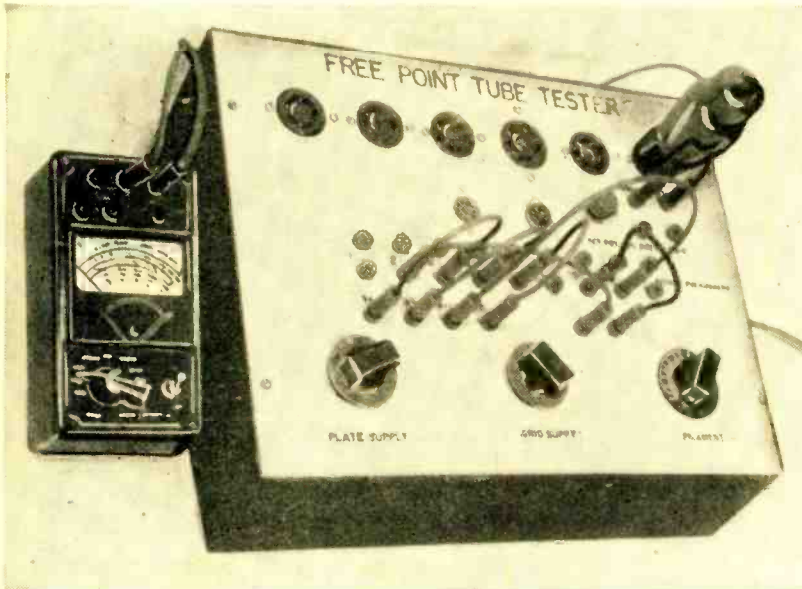
Front view of unit shows sloping panel, with tube being tested. VOM is at left. The author calls his model a "Free Point" tester because all of the socket pins are brought out to corresponding jacks on the front panel which can then be connected to variable plate, grid and filament supplies.
