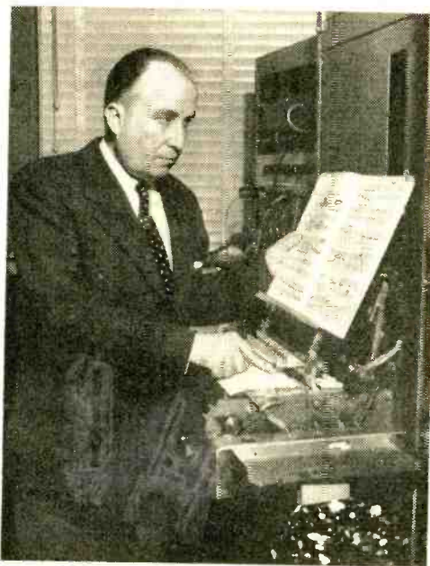
Dr. Olson translates musical score into punched code on "typewriter" keyboard of the Synthesizer (above). The machine converts code to sound recorded by cutter on lower disc (below). Upper disc combines tracks in simultaneous playback.
