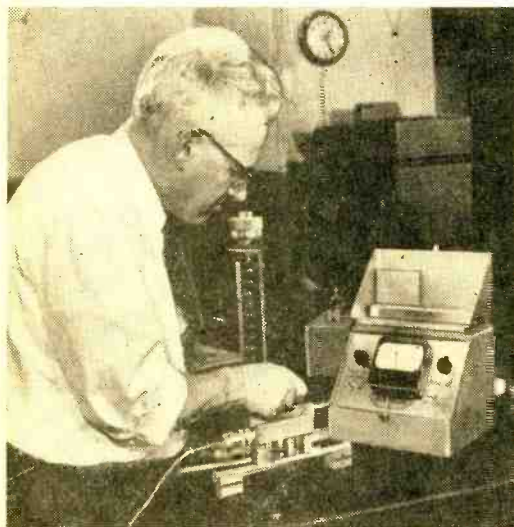
Checking metal parts for proper heat treatment is one of the many duties of the "Metal Monitor." Easy to operate, and requiring no special or technical skill, it is portable and can be moved to the job.
