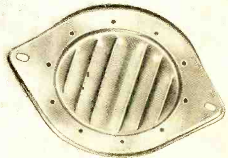
Examples of single-ended electrostatic tweeters are the Arnhold "Isophon" (above) and the Lorenz SKL-100. Both units are small, fairly inexpensive, and simple to connect. Isophon handles range from 7000 cycles and up; Lorenz, 5000 cycles and up.
