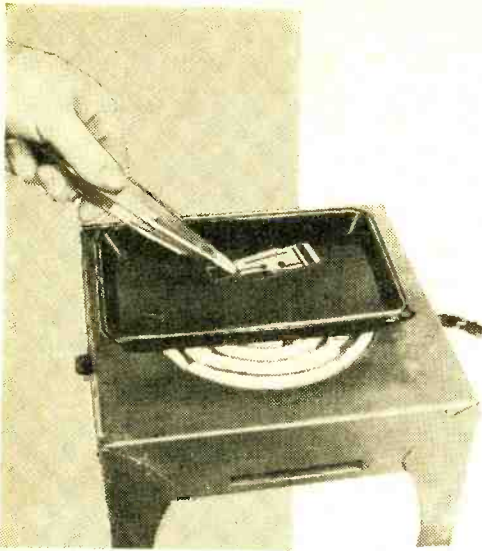
"Hot" method of etching printed circuit board.
