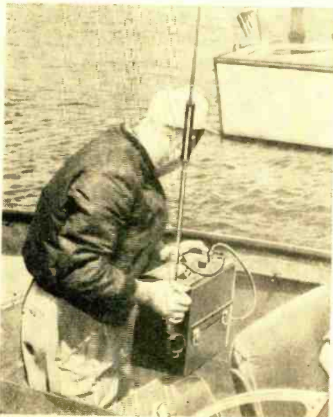
This bag totes a medium-frequency radiotelephone good for a hundred miles under favorable conditions. The "center-loaded" whip antenna telescopes into a socket on the side of the equipment, which is made by Sonar Radio Corporation. Unzip the cover, extend the antenna, connect ground, and you're ready to operate the portable six-channel unit.
