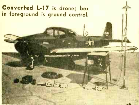
Pictures taken by drone in flight are flashed to television monitor screen. Receiver and ground control unit may be carried in jeep.
