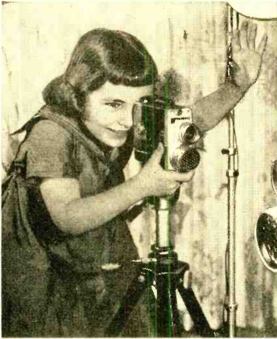
Anyone can shoot movies with this camera. "Electric eye" sets lens at proper exposure and continues to open or close the lens iris as changing light requires. It takes the hard work out of photography.
