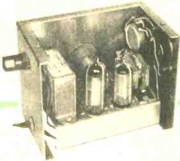
Top left, over-all view of control unit with sensitivity control and a.c. outlet at far left, bull's eye pilot lamp on front. Lower left, inside of cabinet; transformer is at left, relay at right. Top, under-chassis view.
