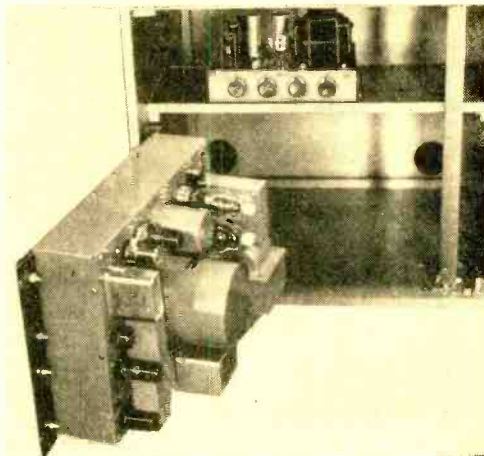
Martin Bender, designer of the console, adjusts output level control during test. Below, bottom view of console, showing how tuning-fork amplifier hinges out for easy accessibility. Smaller amplifier sitting on shelf is used for monitoring.
