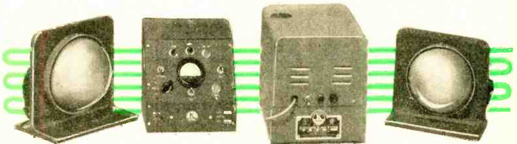
Complete alarm system includes (left to right): transmitter or "speaker," monitor, master control unit, and receiver or "pickup." The combination will detect any motion in a room or other protected area.
