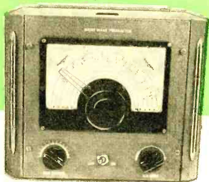
Front view of preselector. Fine tuning control is at left, gain control at right.
