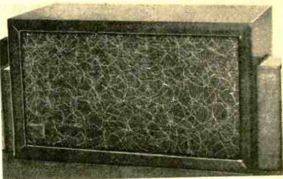
This installation by Fisher Radio uses available closet area for infinite baffle as well as for housing entire hi-fi system.
