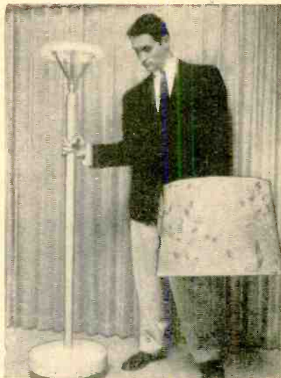
Proud builder and owner holds up his cordless floor lamp. Bulb lights without cord, plug, or socket. Inductive unit located in lamp base operates this unique device.
