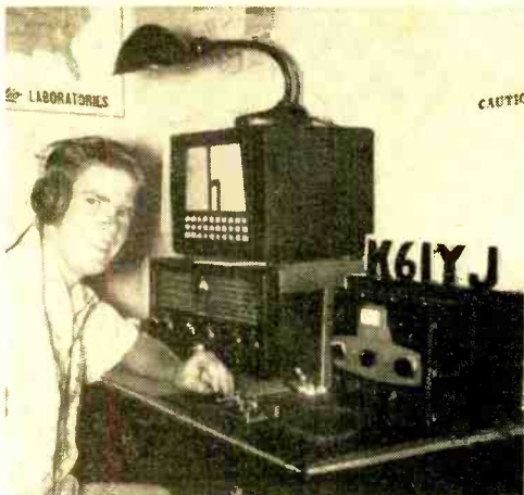
Bill, K6IYJ, (Calif.), has worked 24 states with Johnson "Adventurer" transmitter at 50 watts and Hallicrafters SX-71 receiver.
