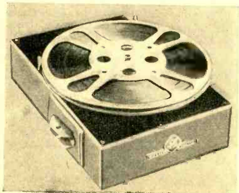
Complete erasure in a matter of minutes is provided by commercial "bulk erasers" such as those shown here. See text for details.
