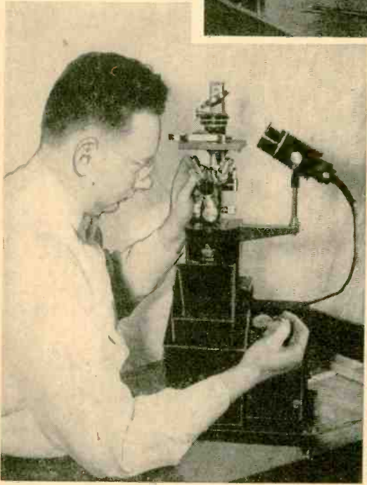
Highly accurate shadowgraph and microscopic studies are made of the finished diamond styli tips.
