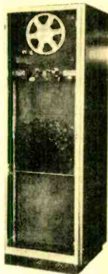
"Datacord," made by Brush Electronics Co., Cleveland, Ohio, is a tape transport mechanism used for high-speed data recording. Tape, loosely stored at bottom, is pulled up by reel. As it passes recording head, data from computers is impressed on it.
